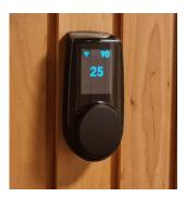
sign will appear when the heater is on. Number in the middle is the current temperature and the smaller one in the corner is the target temperature. Quick double click will toggle the air circulator on/off (a light icon means it is on).
